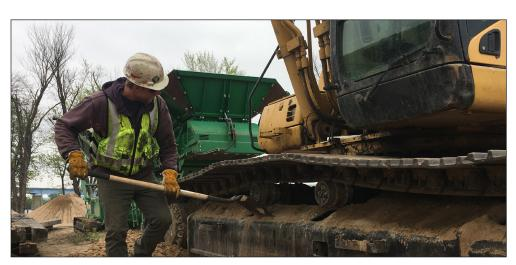
Scott Rolbiecki, operations, removes sand from the tracks of an excavator before dredged material placement at McGregor Lake.
